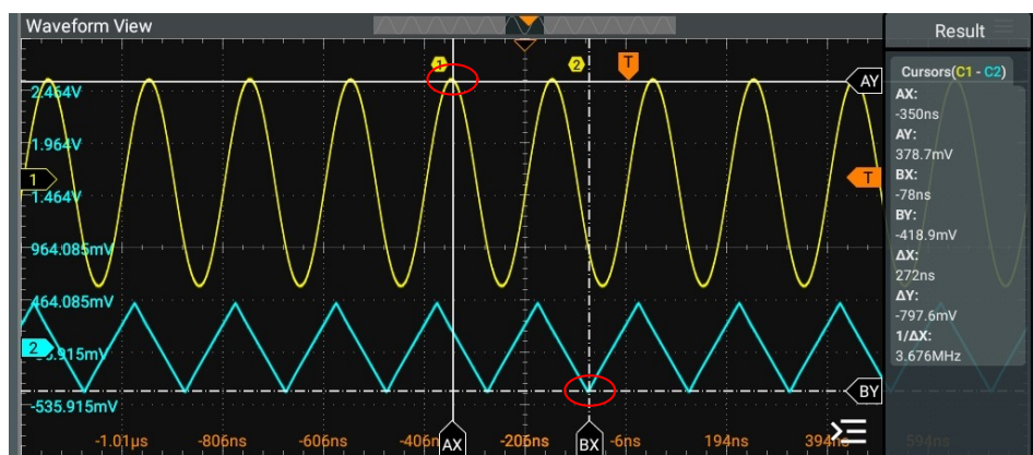
Figure 10.12 Track Measurement (before Horizontal Expansion)
