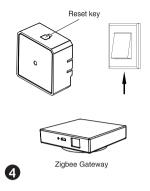
After the wiring of switch module is done, press the reset key for about 10 seconds or turn on/off the traditional switch for 5 times until the indicator light inside the module is flashing quickly for pairing.
