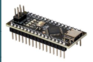
The NanoV4-MC is a particularly small microcontroller and, due to the pin header leading out at the bottom, has been specially developed for working with breadboards.
