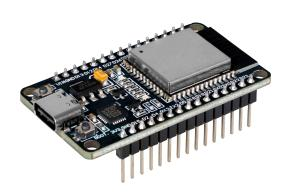
The NodeMCU-ESP32 is an ideal choice for effortless prototyping, offering easy programming through Lua script or the Arduino IDE. Its breadboardcompatible design ensures quick setup and integration into your projects. This powerful development board features 2.4 GHz dual-mode Wi-Fi and BT wireless connectivity, enabling seamless communication for a wide range of applications.
